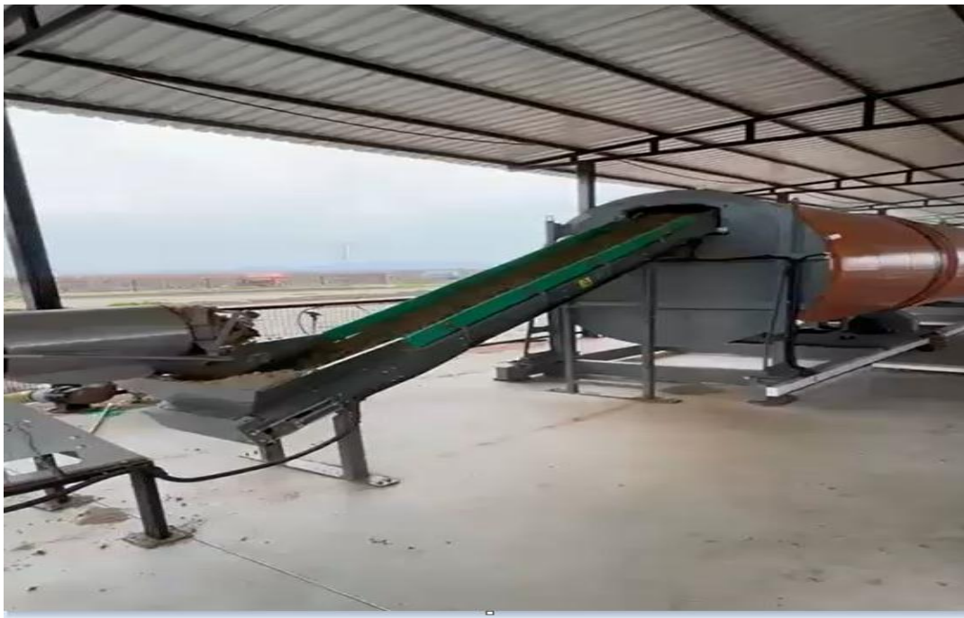
Figure 2: The input to the Bioreactor device (animal manure, waste)
